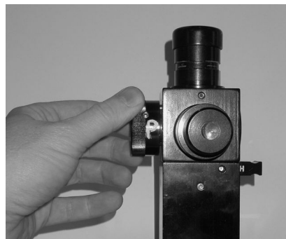
Flipping the mirror: use the fingers, not the wrist
