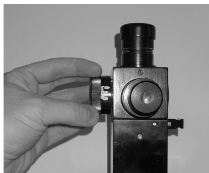
Flipping the mirror: use the fingers, not the wrist
